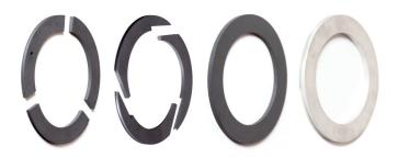
The BTUU ring set includes our latest pressure breaker ring technology. Each seal ring set contains a Radial-cut ring that is single-acting and allows gas to flow out of the cup on suction stroke, a Tangent-cut ring that seals at lower operating pressures, a polymer Uncut ring that seals the leak paths of the tangent cut ring and compresses against the rod at higher differential pressures and a metallic uncut ring that provides structural support for the polymer uncut ring.
